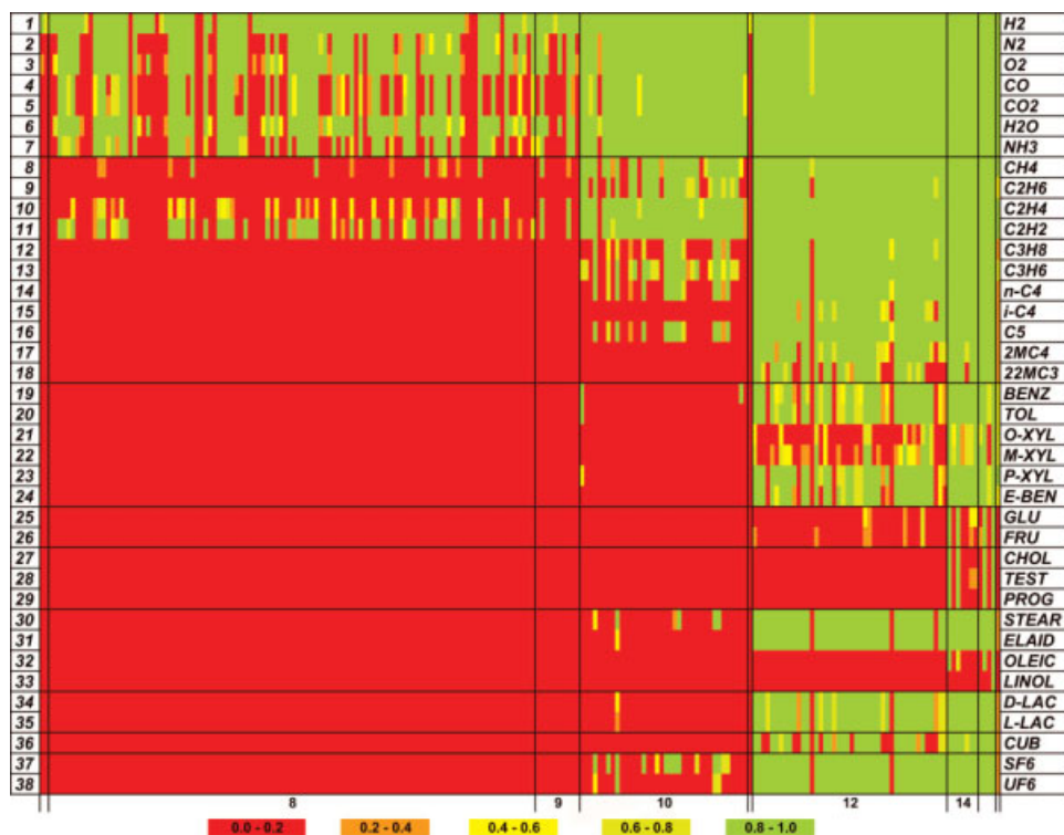
Figure 14. Equilibrium concentration database at T = 300 K (uniform distribution of initial states).
